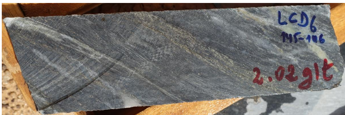
LCD6 core in sulphide-rich mineralized silicified porphyry from Lily.
