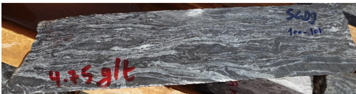
SCD9 core in mineralized quartz-carbonate veined iron-formation from Sophie I & II.
