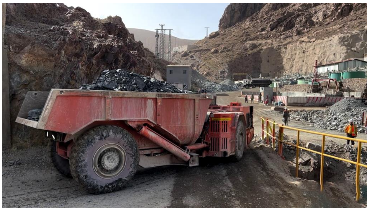
Figure 1 – Six-ton scoop exiting the underground mine
