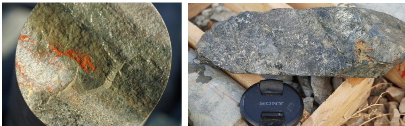
Figure 2: Silver rich proustite mineral coating fractures (left). Native silver on core (right).
